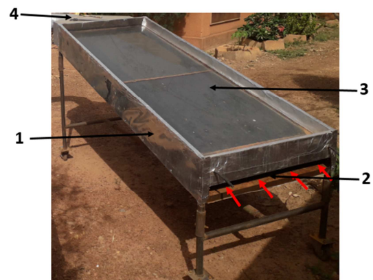
Figure 2. Experimental device. (1) Collector, (2) Enter air, (3) Glass, and (4) Extractor.
